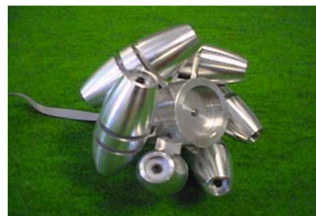
Figure 9.1: Mecanum wheel designs with rollers at 45^\circ
