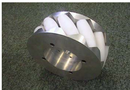
Figure 9.1: Mecanum wheel designs with rollers at 45^\circ
